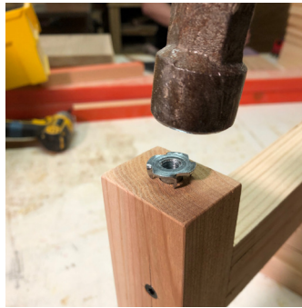
Place the leveling foot base in the hole and hammer until flush. Screw in the feet.
