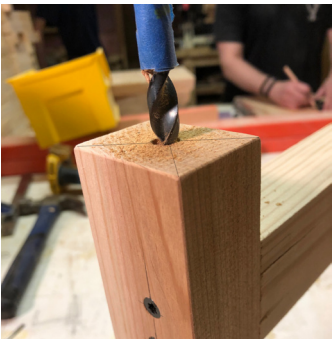
Mark and punch with nail set the center of legs. Pre-drill a hole (max 1" deep) with 3/8" bit.
