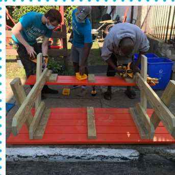
Grab a friend and all your clamps. Attach seats to seat braces.
