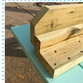
Align 9 ½" blocks of seat to edge of seat braces of legs.
