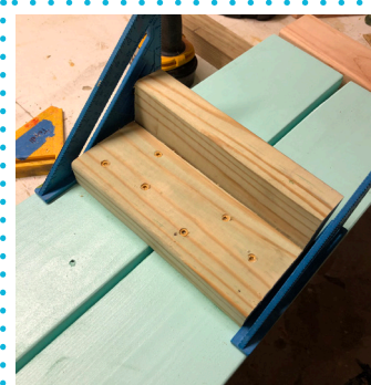
Attach with 2 1/2" screws in a zig-zag pattern. 3 screws per slat. Remember to pre-drill.
