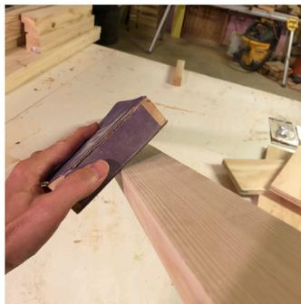
Chamfer (angle) all corners with a sanding block to create comfortable edges.
