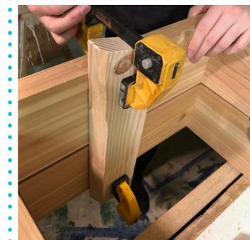
Clamp 2 or 3 pieces of scrap wood along inside surface to align rings.
