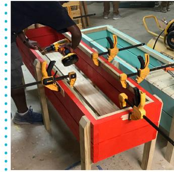
Install ledger strips on top of plastic and flush to top of planter.
