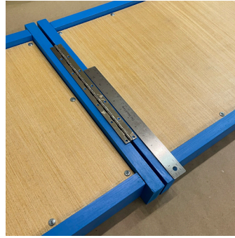
Position two sign pieces with the tops \frac{1}{4} " apart, and place hinge in the center.
