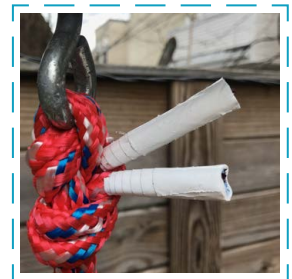
Tape or melt rope ends
