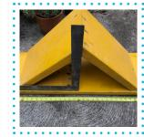
Use the framing square to align the triangle base with the middle of the length of the seatboard
