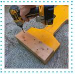
Pre-drill 2 x 4 seat reinforcers, glue, align and screw to seatboard. Sand and paint everything!
